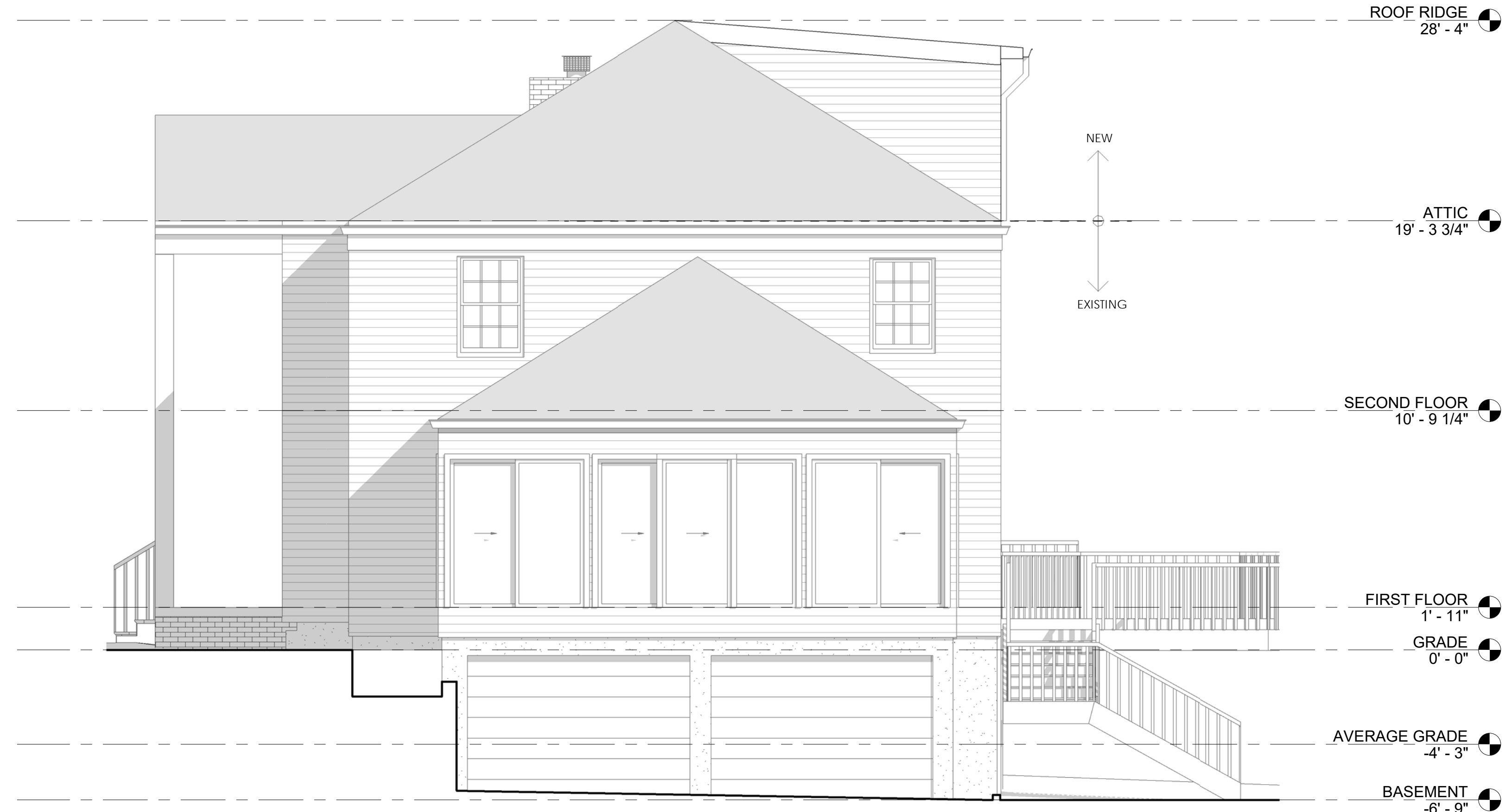
2 RIGHT SIDE ELEVATION - NEW CONSTRUCTION 1/4" = 1'-0"
